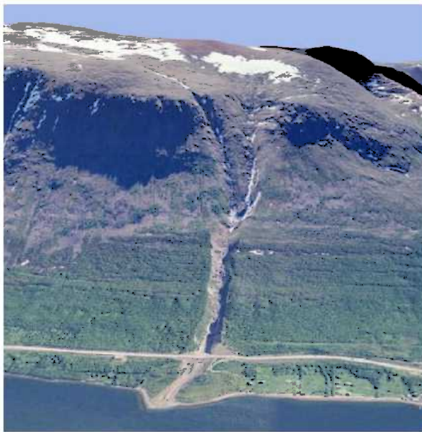
Fig. 11: Herraneselva, Langfjorden, Alta, North Norway, 19.05.2000. a) The mountainside with the two slushflow paths. Starting zones in the high-lying basins. The bridge is replaced by a fill after the bridge was lost in the fiord in 2000. ( www.kart.finn.no ) b) The crossing after the bridge was gone. It is an 800 km detour via Finland from one side to the other.
