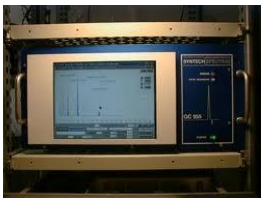
Figure 4: For monitoring of Benzene-Toluene-Xylene (BTX) components a Syntech Spectras GC-855 (Synspec, Groningen, The Netherlands) monitoring device was used. Figure reproduced with courtesy of Synspec, Groningen, NL
